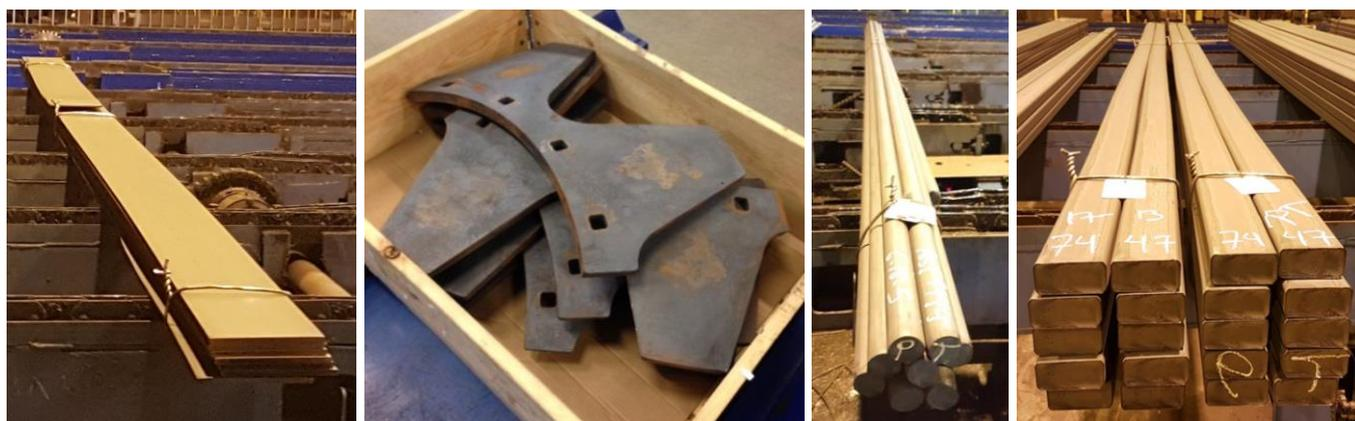
Four examples of steel produced in project "AusFerrit": Ingot rolled to flat bar 200×10 mm, steel castings "Grating teeth" after austempering heat treatment, ingot rolled to round bar  $\varnothing 53$  mm, and continuous cast billets rolled to spring steel profile 95×49 mm
